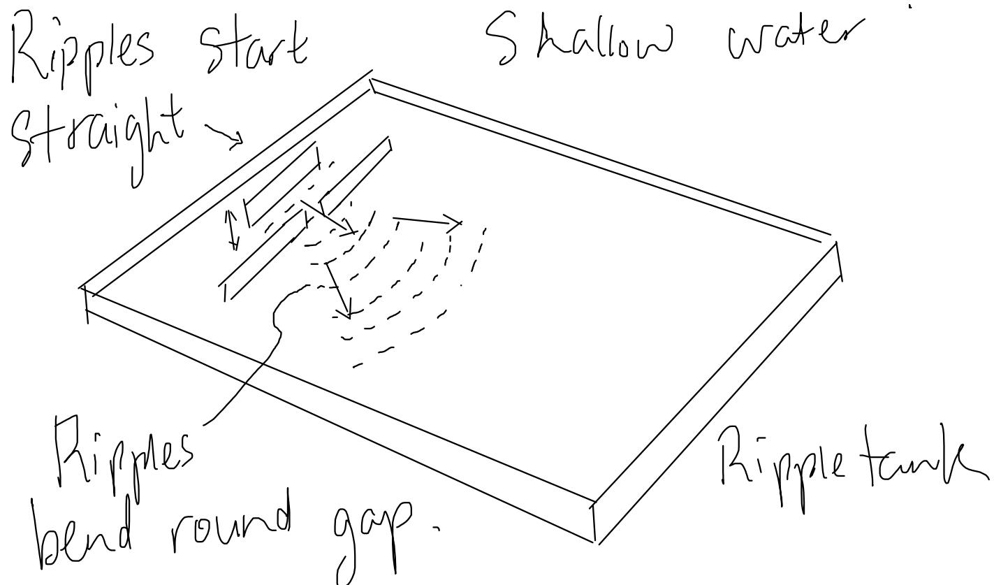
Diffraction - Wave bending round corner.
